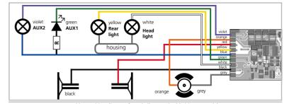
Abb. 4: Wiring diagram for LokPilot Standard (wiring example)
